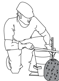
Figure S. Slump Test (Measurement)
